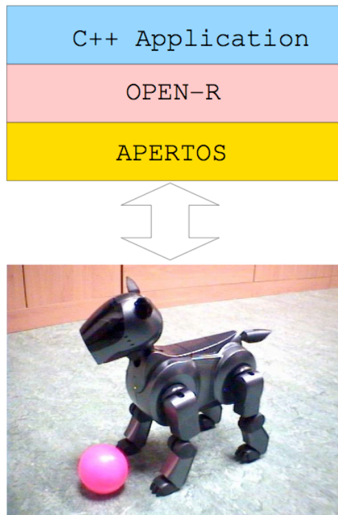
Fig 5. Software architecture for programming Sony Aibo robot
