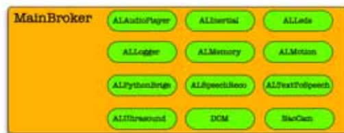
Fig. 3. Modules within MainBroker.
