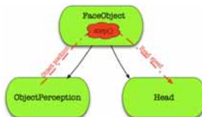
Fig. 12. Activation tree with two low level components and a high level component that modulates them.
