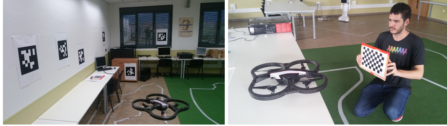
Fig. 2. Real ArDrone2 and calibration of its onboard camera
