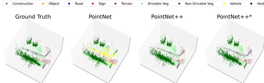
**Fig. 5.** Qualitative comparison of semantic segmentation results on a GOOSE test point cloud not used for model training. Class labels are shown at the top.
