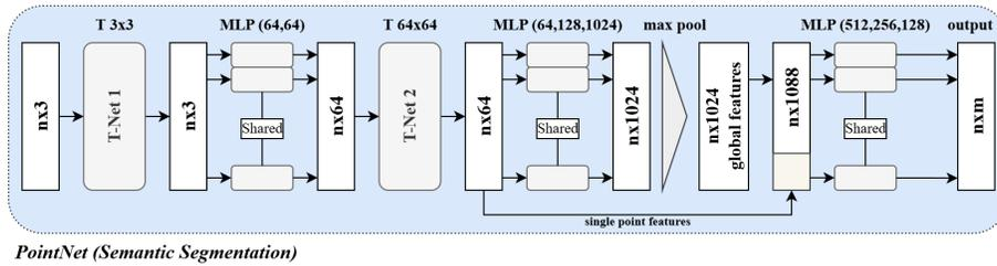
**Fig. 2.** Block diagram of the PointNet architecture.
