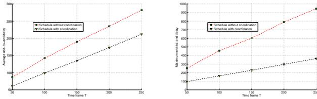
Fig. 1. Average (left) and maximum (right) end-to-end delay for a line network of length 40, with 50 connections of path length 10.
