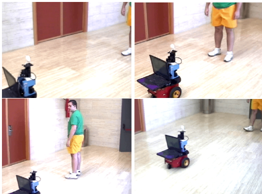
Figure 7: Robot keeps the distance using only vision
