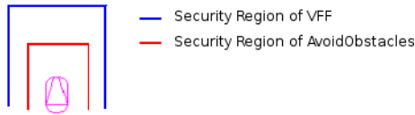
Figure 4: Security region for VFF and avoid-obstacles schemas
