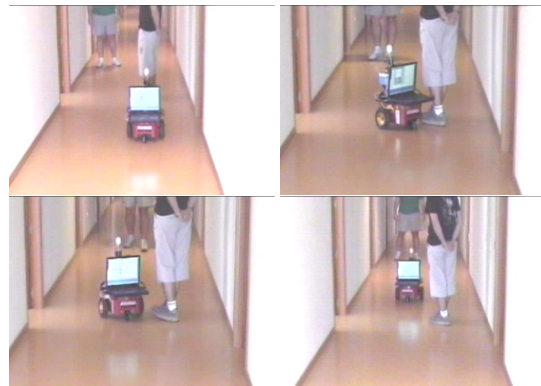
Figure 5: Obstacle avoidance while pursuing target
