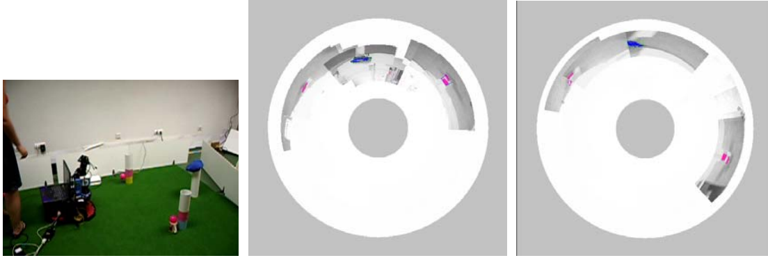
Figure 8. When the robot approaches to the objects, they spread out in the image scene.
