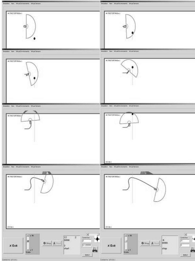
**Fig. 7.** Robot trajectory (black) described by the activation of only three rules from the AVOID strategy, due to the lack of knowledge on the moving object. Vehicle and obstacle speed are 0.3 and 0.5 m/s, respectively. Object trajectory is represented by a grey straight line, and semicircles limit the emergency areas.
