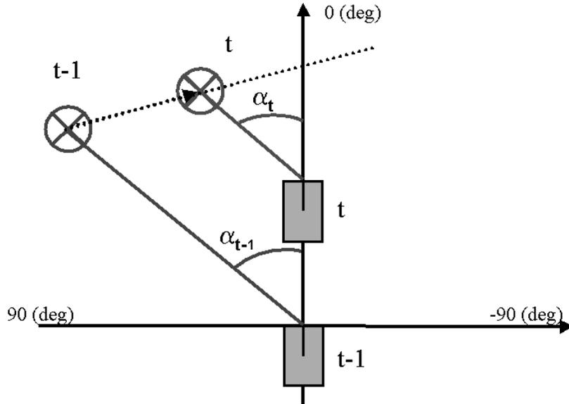
**Fig. 2.** Collision\_angle  $\alpha$ , in  $t$  and  $t - 1$ , measured with respect to the vehicle heading. Constant values of the *collision\_angle* variable in a time period indicates collision risk
