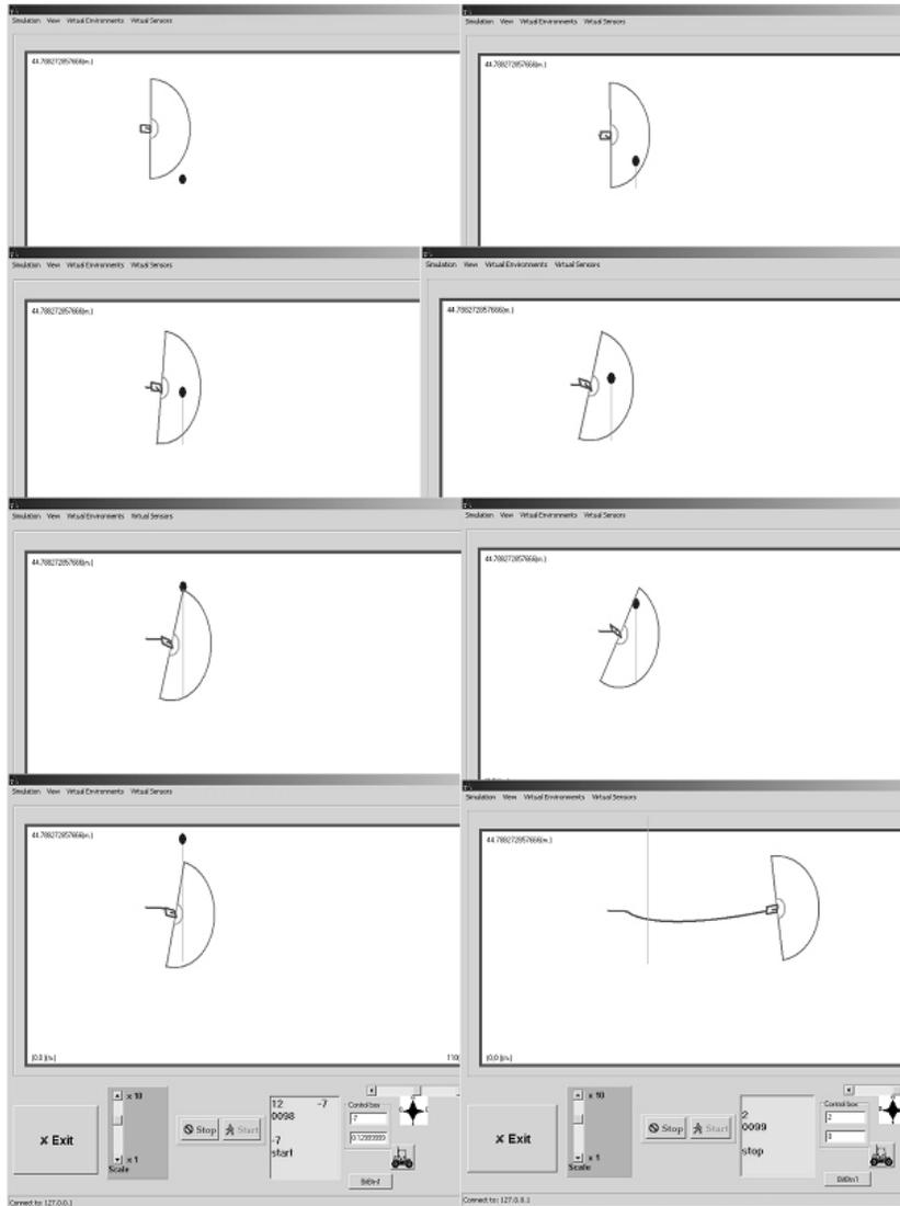
**Fig. 8.** Robot (black) and object (grey) trajectories. Deviations from the robot goal-driven tentative trajectory are optimised due to the existing knowledge on moving object descriptors. Vehicle and obstacle speed are 0.3 and 0.5 m/s, respectively.
