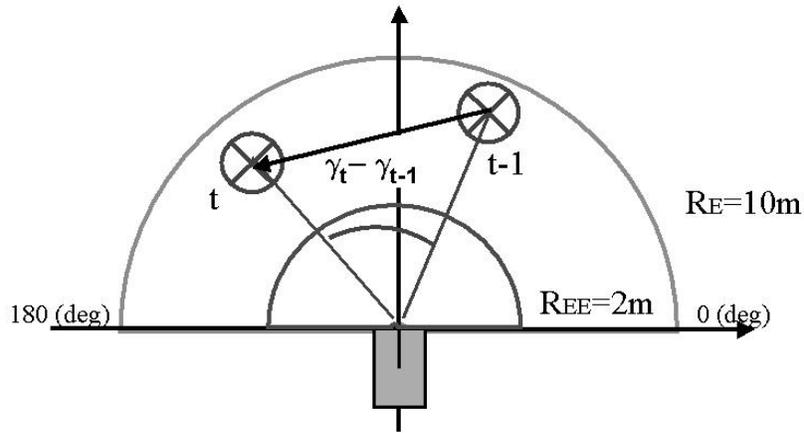
**Fig. 4.** Inputs to the AVOID strategy : $\gamma(t)$  moving object angular distance in  $t$ , relative to a laser-centred reference system, and  $[\gamma(t - 1) - \gamma(t)]$  angular distance variation of the moving object location in two successive steps.  $R_{EE}$  is the radius of the extreme emergency zone, while  $R_E$  corresponds to the emergency area
