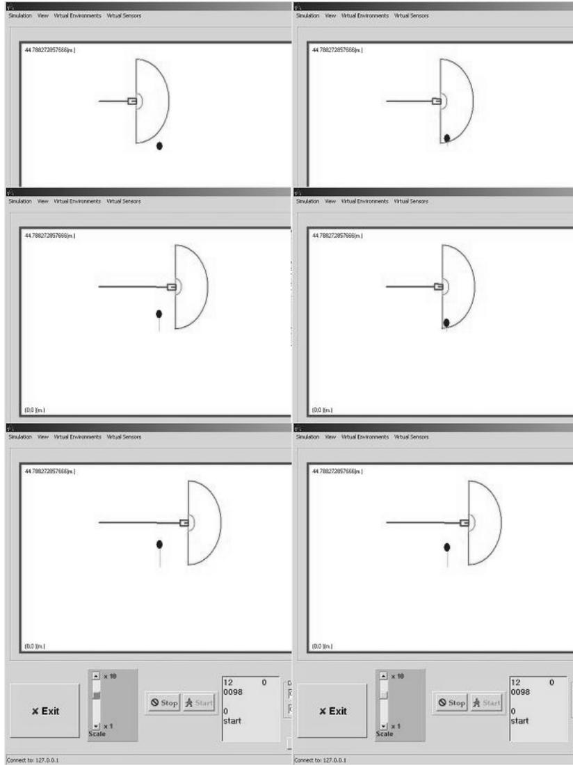
**Fig. 10.** Robot (black) and object (grey bottom-up) straight line trajectories. Optimized robot trajectory in the presence of an object in the emergency area. No detour is performed as there is no collision risk ( $v_{robot} = 0.3$  m/s,  $v_{object} = 0.05$  m/s).
