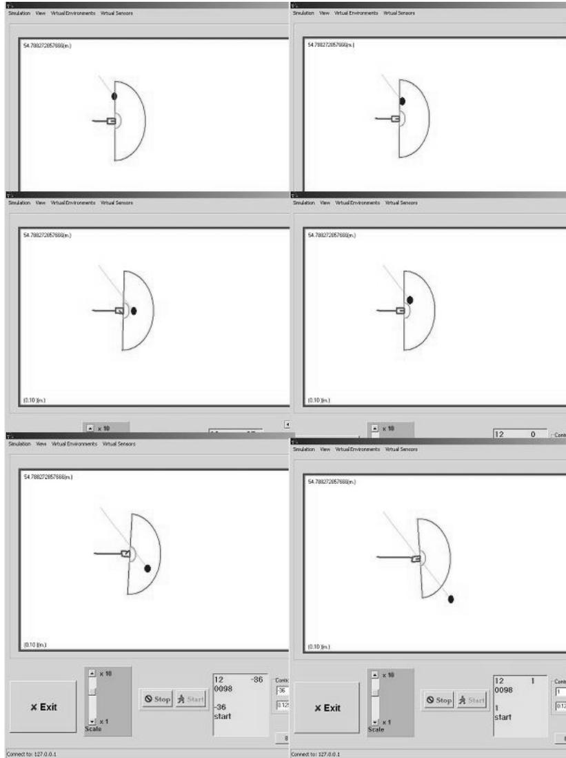
**Fig. 9.** Robot (black) and object (grey) straight line trajectories. The AVOID agent is not activated as collision risk is not detected, in spite of a speedy object is within the emergency area. ( $v_{robot} = 0.3$  m/s,  $v_{object} = 0.5$  m/s).
