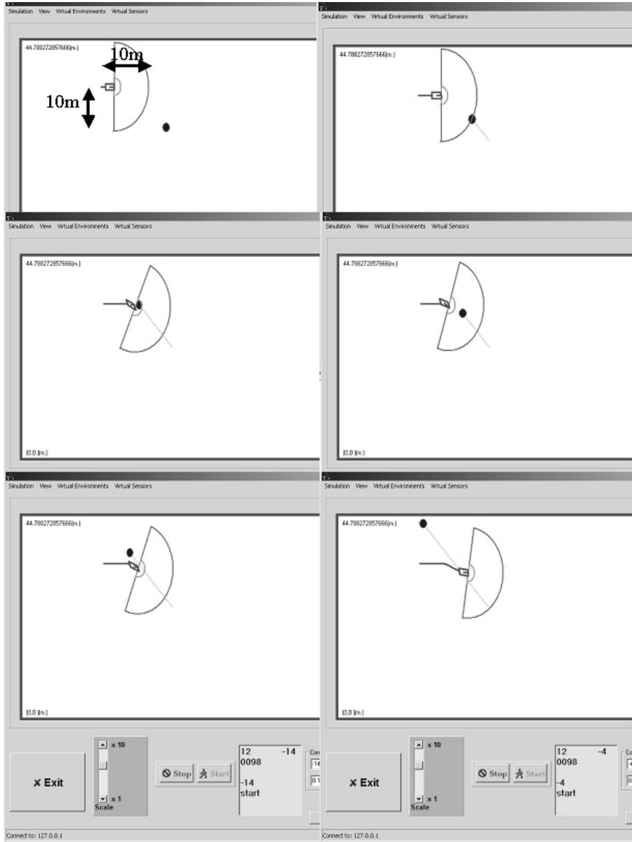
**Fig. 3.** Robot (black) and object (grey straight line) trajectories. The goal-driven robot trajectory is slightly deviated from its target through the activation of the AVOID strategy as collision risk is detected. ( $v_{robot} = 0.3$  m/s,  $v_{object} = 0.5$  m/s).
