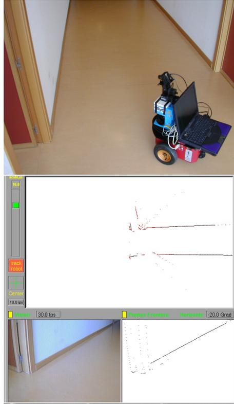
Figure 3: Robot facing to the wall, monocular and edge images, and visual memory
