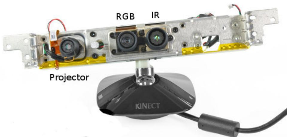
FIGURA 3.1: Sensor Microsoft Kinect
