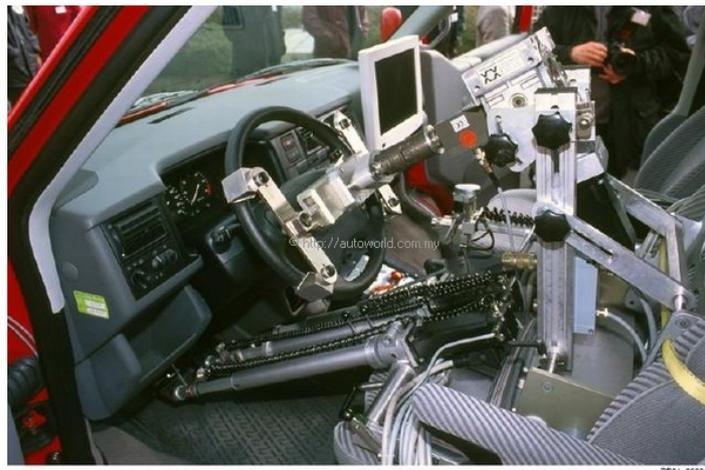
Figura 1.2: Robot conductor Klaus.
