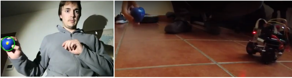
Figure 4.28: Navigation exercise of following a color object using vision in PiBot
