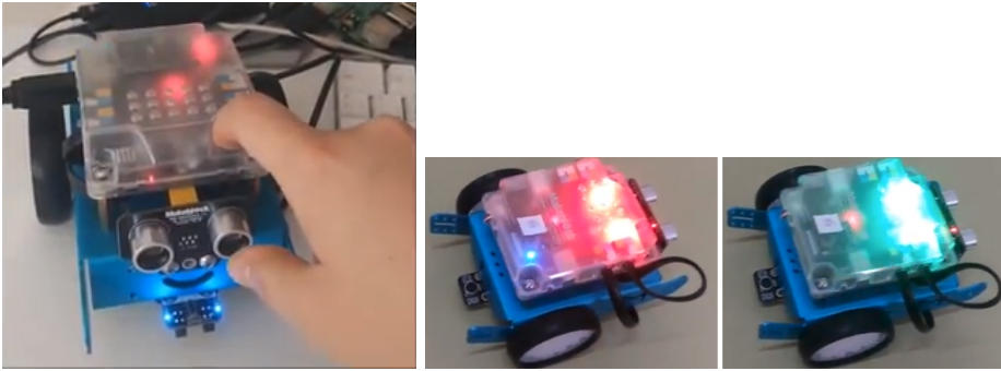
Figure 4.17: Practice tasks with mBot to operate push-button and LED, and microphone with LED to recognize sounds
