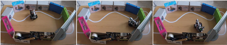
Figure 4.27: Navigation practice avoiding obstacles through US in PiBot
