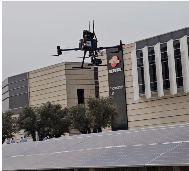
Figure 5.8: DJI M300 inspecting a PV plant at the Repsol Technology Lab in Móstoles, Madrid.
