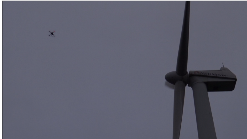
Figure 5.1: Autonomous wind turbine inspection at Sotavento, Lugo.
