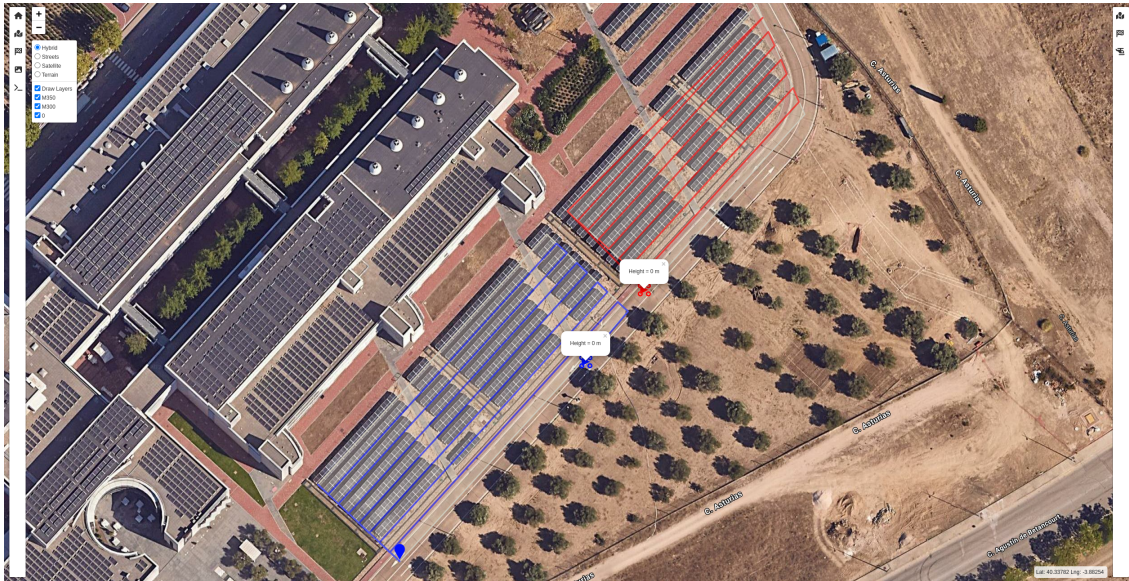
Figure 5.11: Area coverage mission definition using Aerostack2 webGUI.
