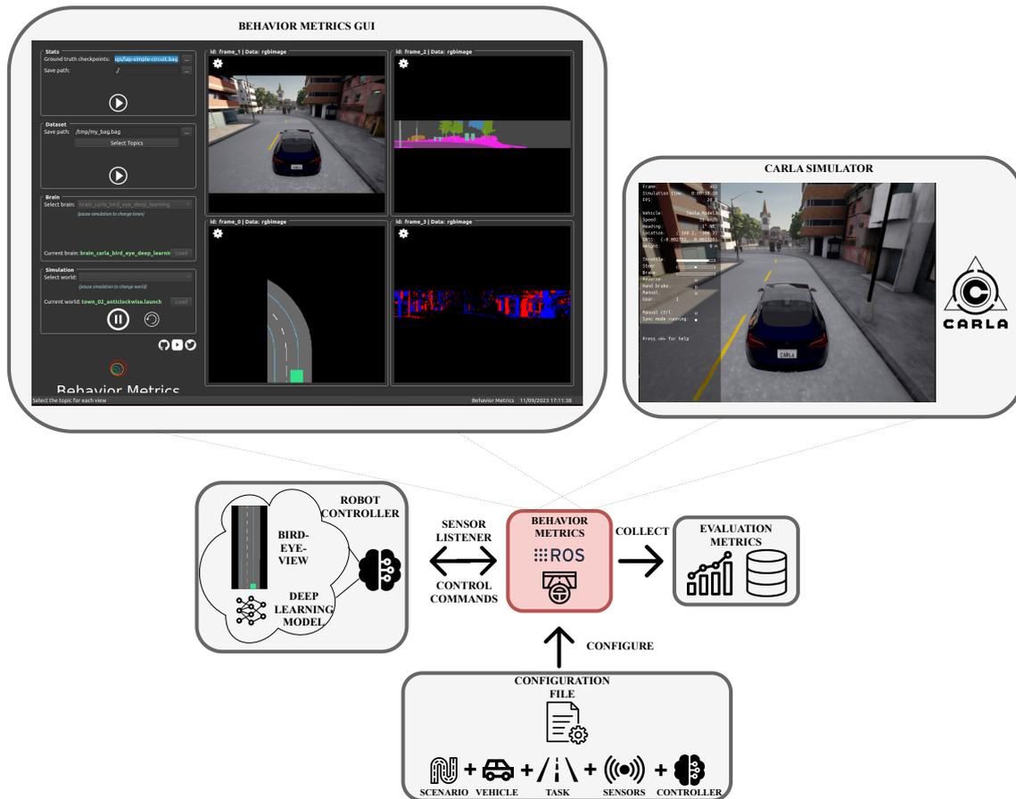
Figure 5.4: Behavior Metrics GUI architecture using CARLA simulator. It displays two separate windows: the application GUI and the simulator.
