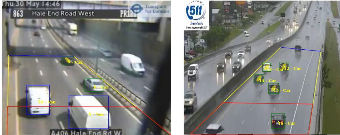
Figure 3.18: *TrafficSensor* with poor resolution (left) and bad weather (right) videos.
