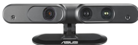
Figure 3.3: Asus Xtion Pro Live. IR emitter (left), and RGB and IR lenses (right).
