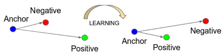
Figure 6.6: Triplet loss training. It minimizes the distance between an anchor (current example) and a positive , both of which have the same identity, and maximizes the distance between the anchor and a negative of a different identity (from [5]).
