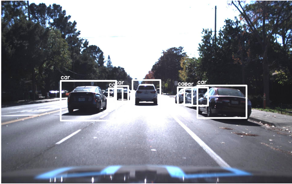
Figure 6.1: Vehicle detection with YOLO applied to Udacity’s self-driving car dataset (source [33]).
