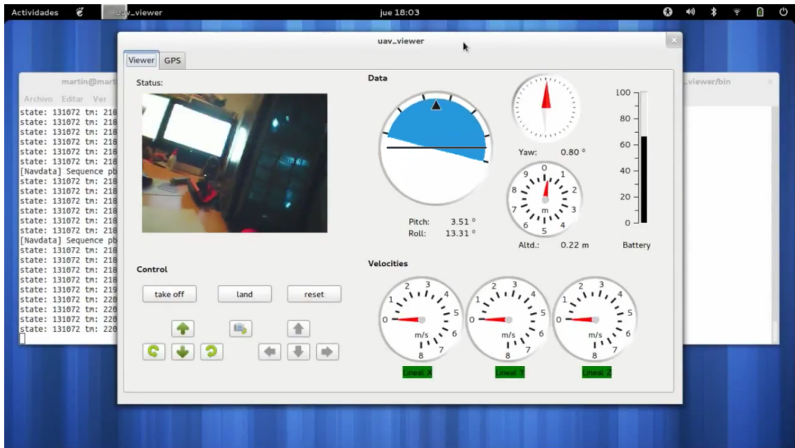
FIGURE 5.3: Uav-viewer connected to Hoverwasp trough MAVLinkServer
