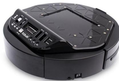
Figura 3.3: Base kobuki. Imagen obtenida de [Robosavvy, 2022]
