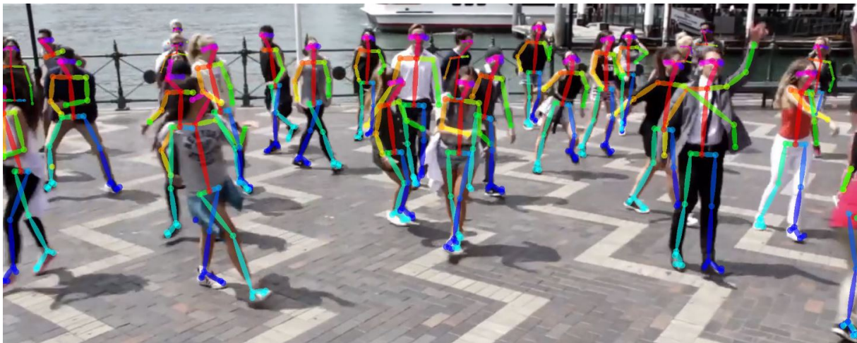
Figure 1.3: Multi-person 2D poses estimated by OpenPose system in real-time [13].
