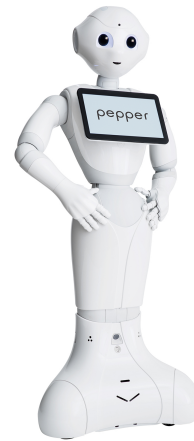
(b) Pepper, an autonomous humanoid capable of performing on-board processing and reacting to external stimuli intelligently.
