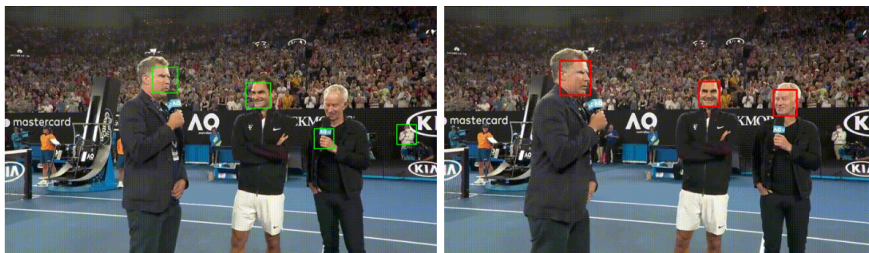
Fig. 2.18. Classical Haar based face detector [12] (left) vs. faced (right). Image from [34].
