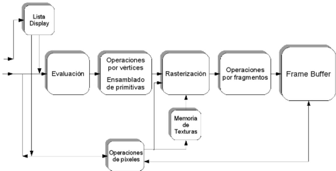
Figura 3.3: Pipeline de OpenGL.
