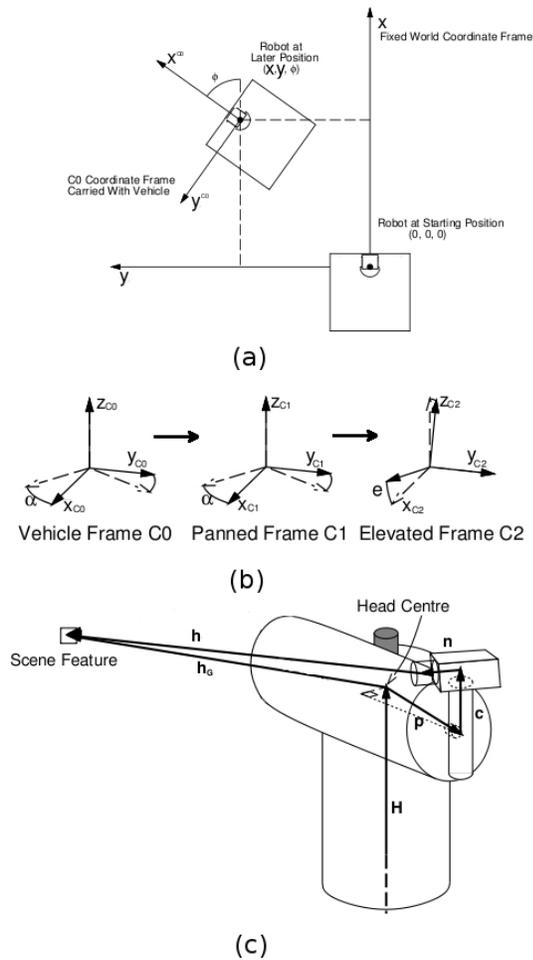
Fig. 6. Coordinate systems used to define the geometric model
