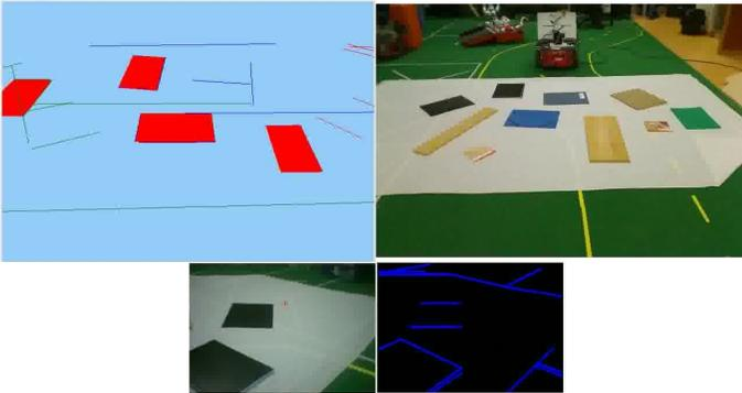
Fig. 12. Parallelograms recognition. Final stage
