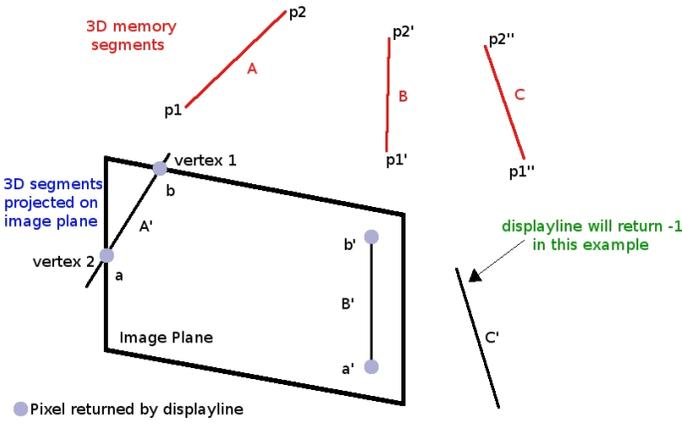
Fig. 3. Segments projection onto the image plane
