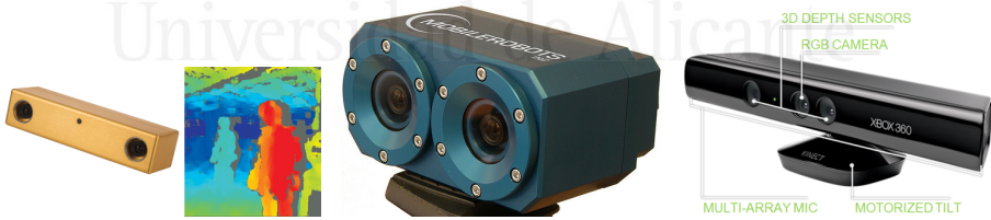
Figure 1.5: Advanced systems of Visual perception: Bumblebee, Mobile Ranger and Kinect
