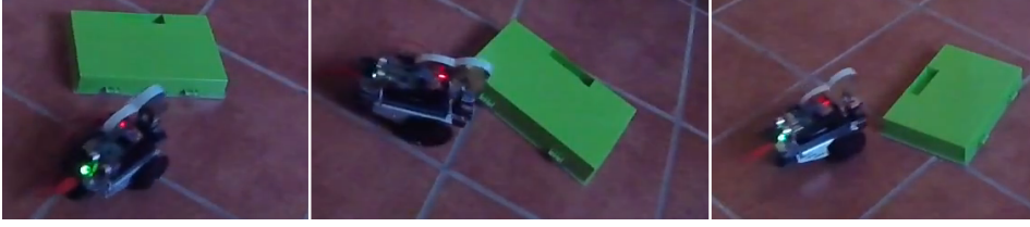
Figure 4.30: Exercise of avoiding obstacles by visual depth estimation in PiBot
