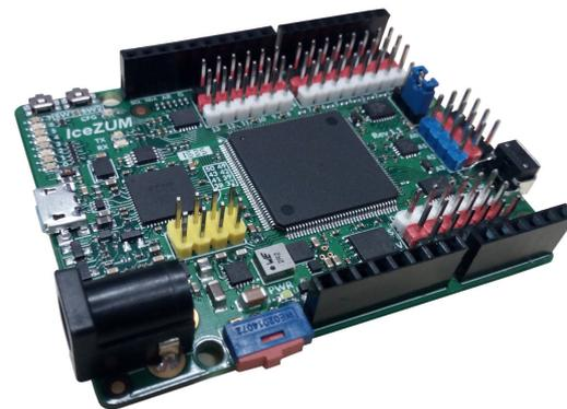
**Figure 2.** IceZUM Alhambra FPGA board.
