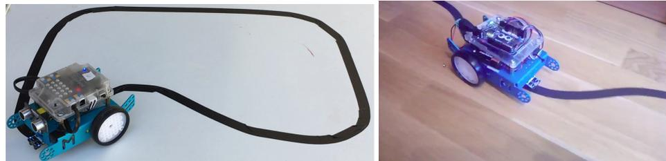
**Figure 7.** mBot robot following a line with a reconfigurable computing brain (left) vs. with a software brain (right).
