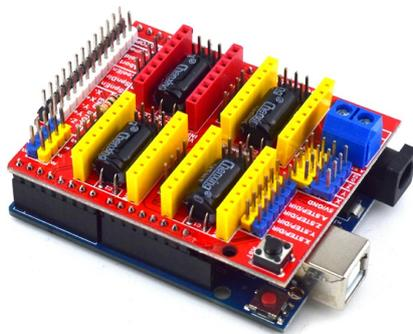
(a) Arduino Uno CNC Shield
