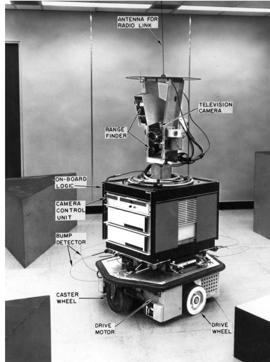
Figura 1.2: Robot Shakey
