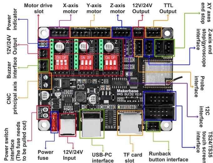
Figura 4.6: Placa base MakerBase DLC32
