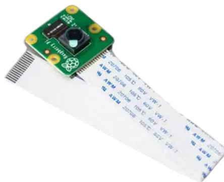
Figura 4.2: Raspberry PiCamera V2<sup>26</sup>
