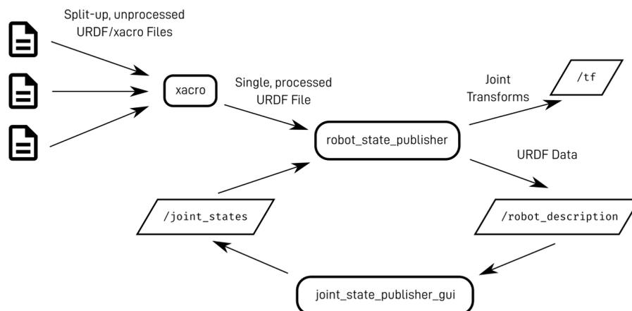
Figura 6.3: Diagrama de robot\_state\_publisher
