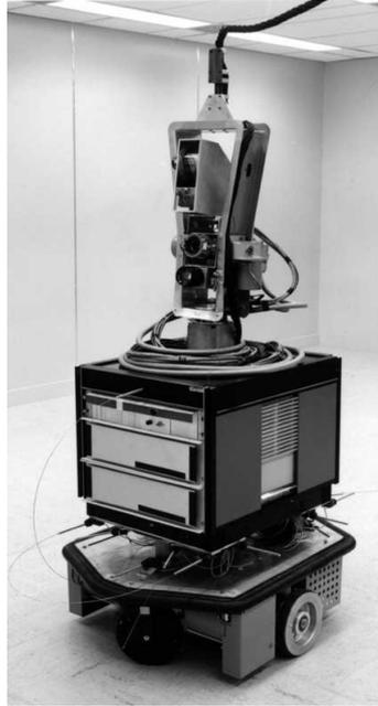
Figura 1.2: Robot Shakey.
