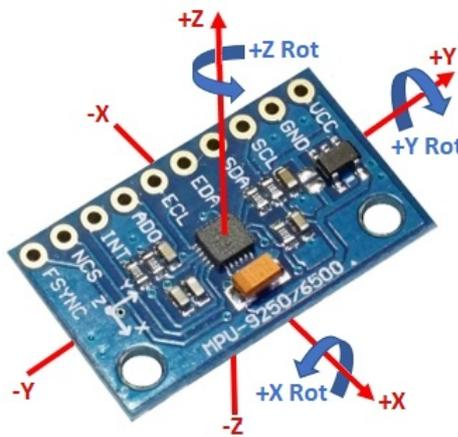
Figura 4.10: Sensor MPU9250.
