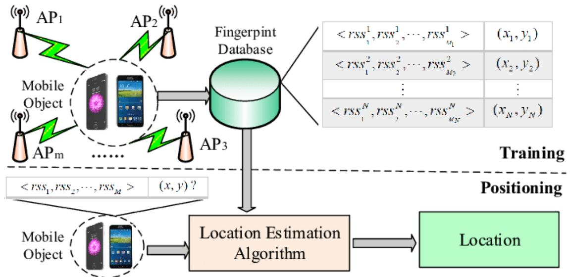
Figura 2.2: Principio de WiFi fingerprinting.
