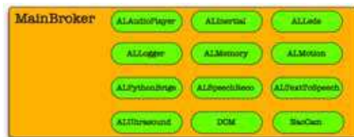
Fig. 3. Modules within MainBroker.
