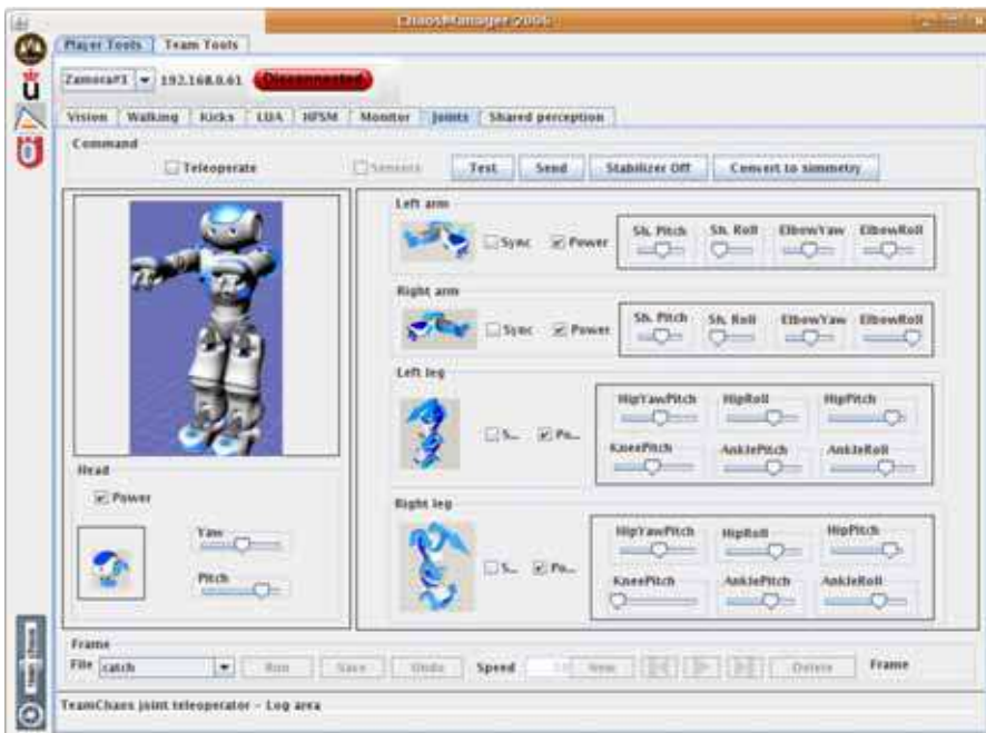
Fig. 28. Fixed movement sequence generation tool.
