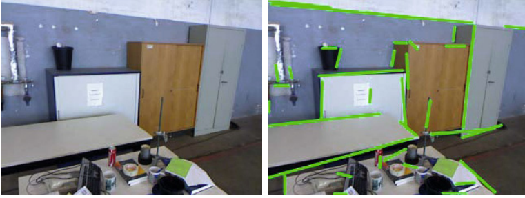
Fig. 3. Line detection in an indoor scenario, 36 lines detected in 4.5 ms
