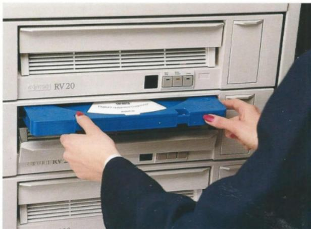
Digital's RV20 laser drive and RV02 media, a fully integrated storage subsystem for the VAX environment, is the first member of a Digital product family based on the rapidly maturing write-once-read-many (WORM) optical technology.
