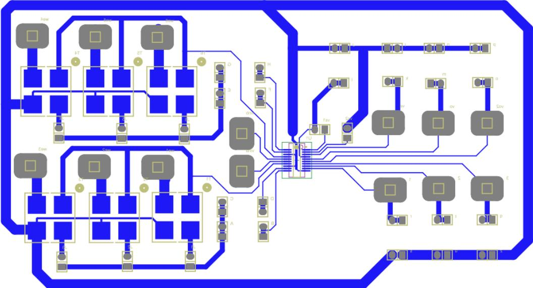
Figure 4.29: Welding simulation LTC3109 circuit
