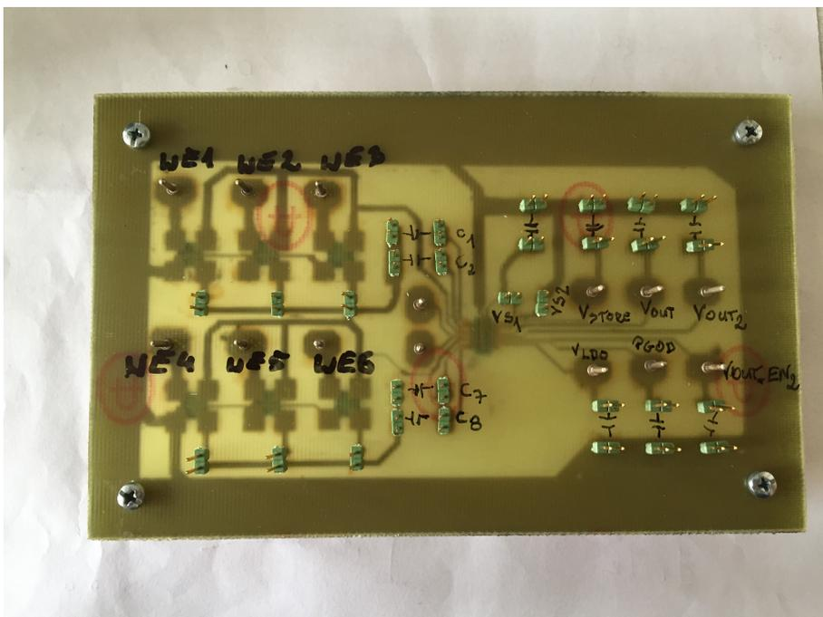
Figure 5.25: Welded Top Board for LTC3109
