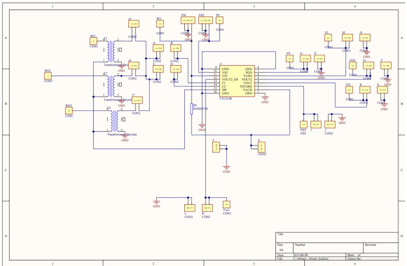
Figure 4.26: Scheme of LTC3108 circuit
