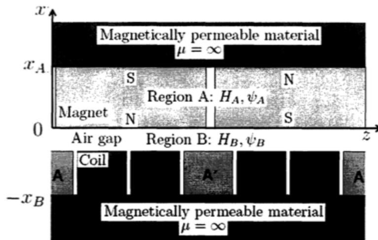
Figure 2.3: Magnet-across-coils induction system
