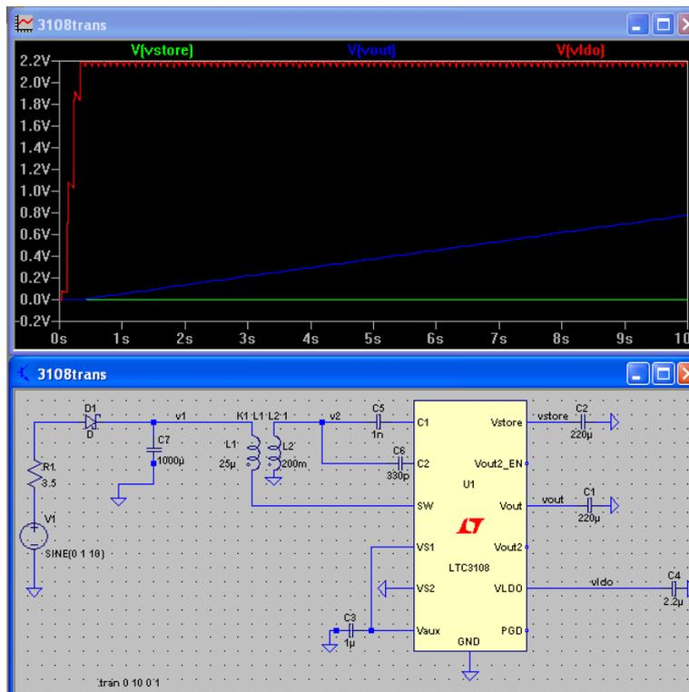
Figure 5.13: Half Wave Rectifier Circuit 5
