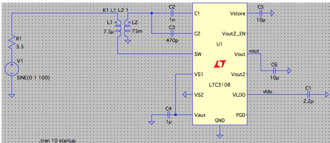
Figure 4.23: Simulation circuit ratio 1:100
