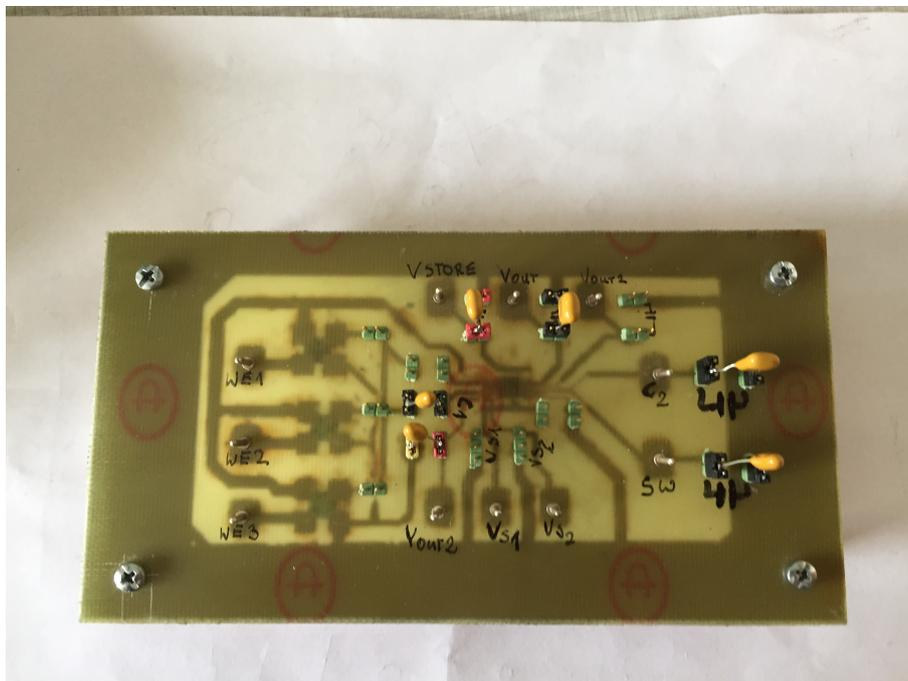
Figure 5.23: Welded Top Board for LTC3108
