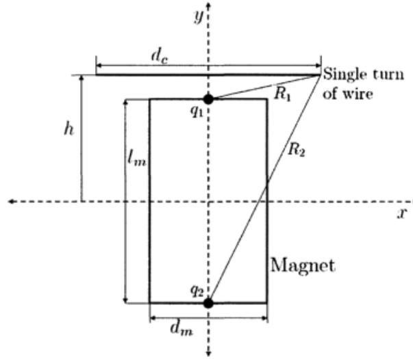
Figure A.3: Magnetic dipole and single wire turn geometry.
