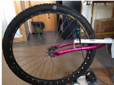
Figure 4.12: Magnets on the wheel
