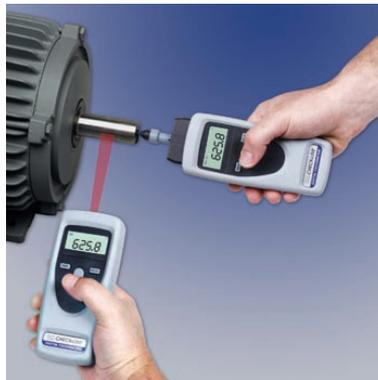
Figure 4.3: Tachometer
