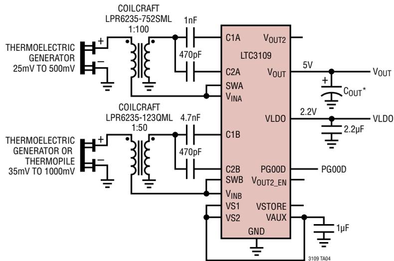
\*THE VALUE OF THE  $C_{OUT}$  CAPACITOR IS DETERMINED BY THE LOAD CHARACTERISTICS
