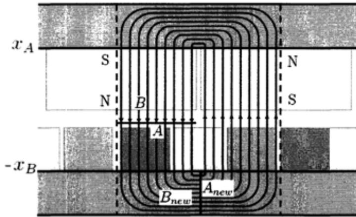
Figure A.7: Path of the magnetic flux in a magnet-across-coils system.
