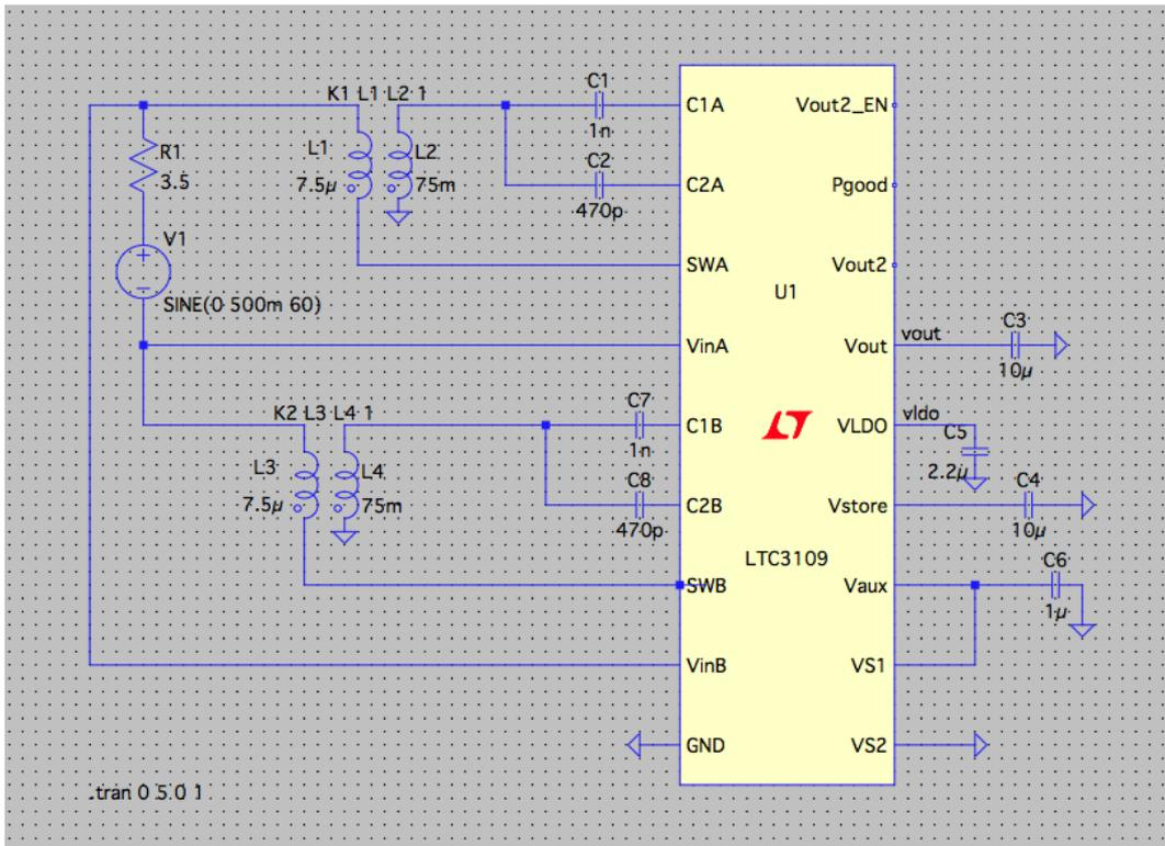
Figure 4.24: Simulation with LTC3109
