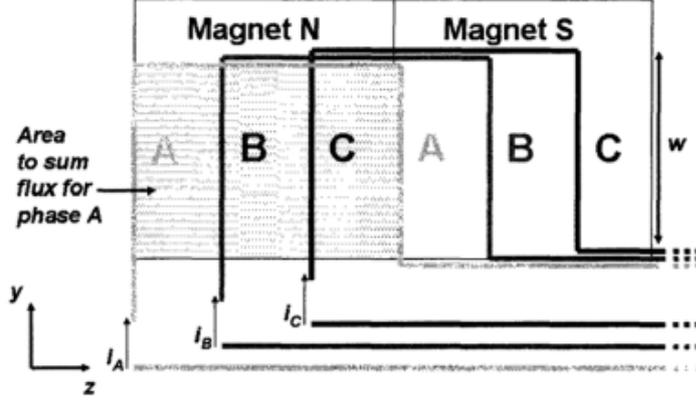
Figure A.6: Three-phase coil arrangement geometry.
