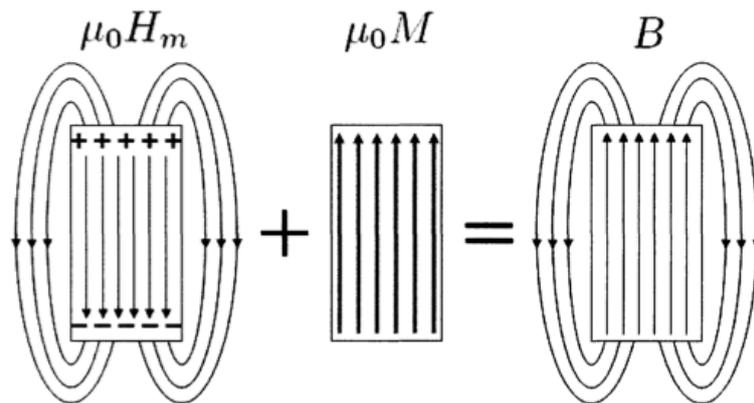
Figure A.1: Magnetic flux density from a bar magnet.
