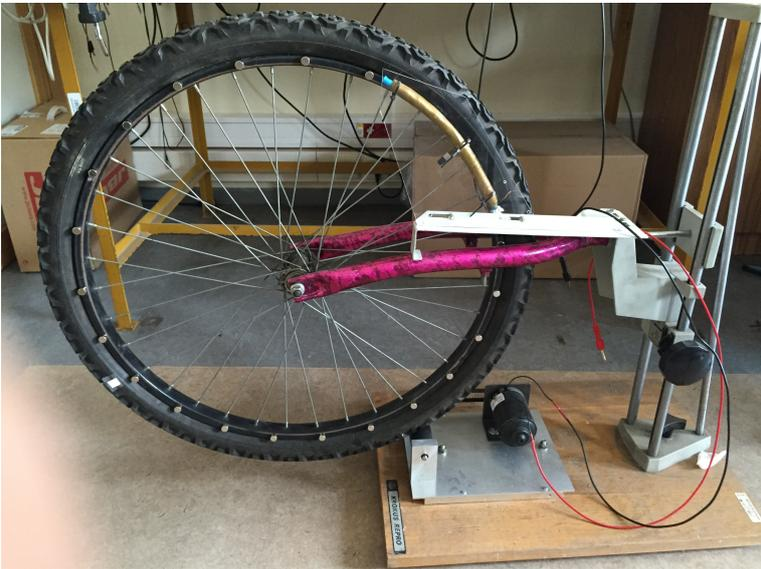
Figure 4.21: Homemade coil attached to the prototype
