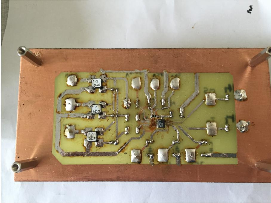
Figure 5.24: Welded Bottom Board for LTC3108
