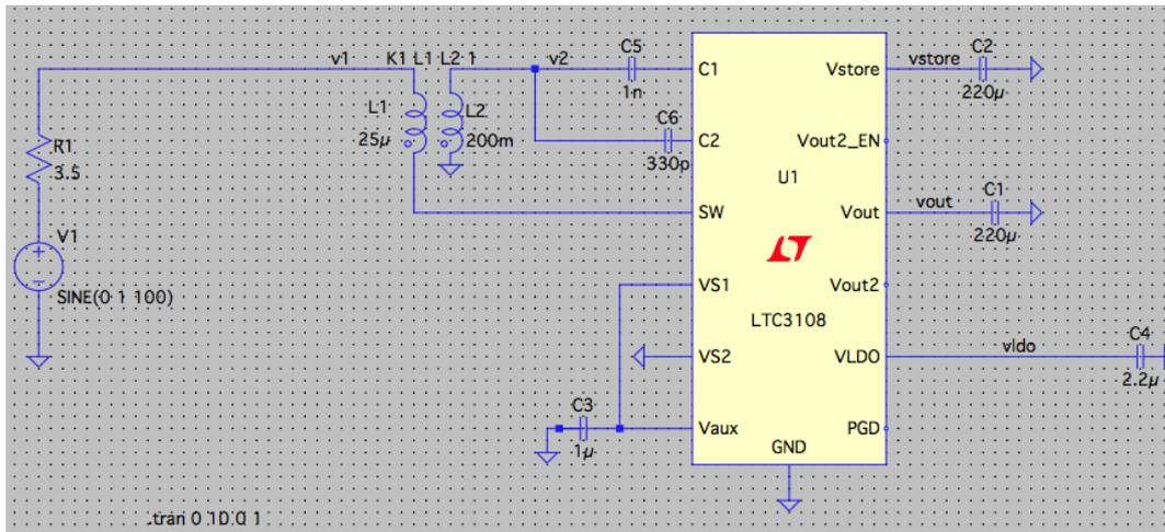
Figure 4.22: Simulation circuit ratio 1:20
