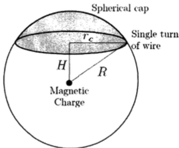
Figure A.2: Point charge and single wire turn geometry
