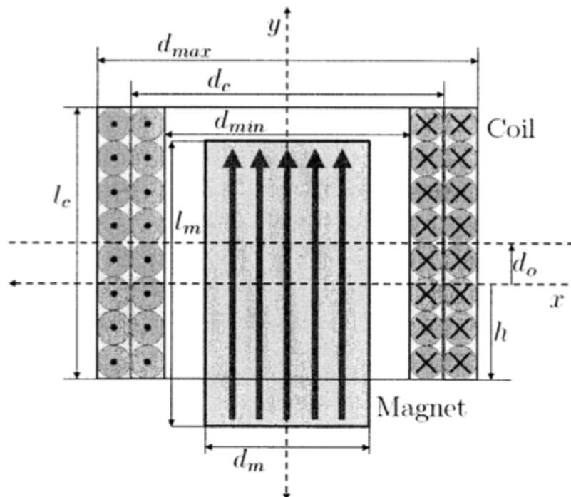
Figure 2.2: A cross-sectional view of the magnet-through-coil induction system.
