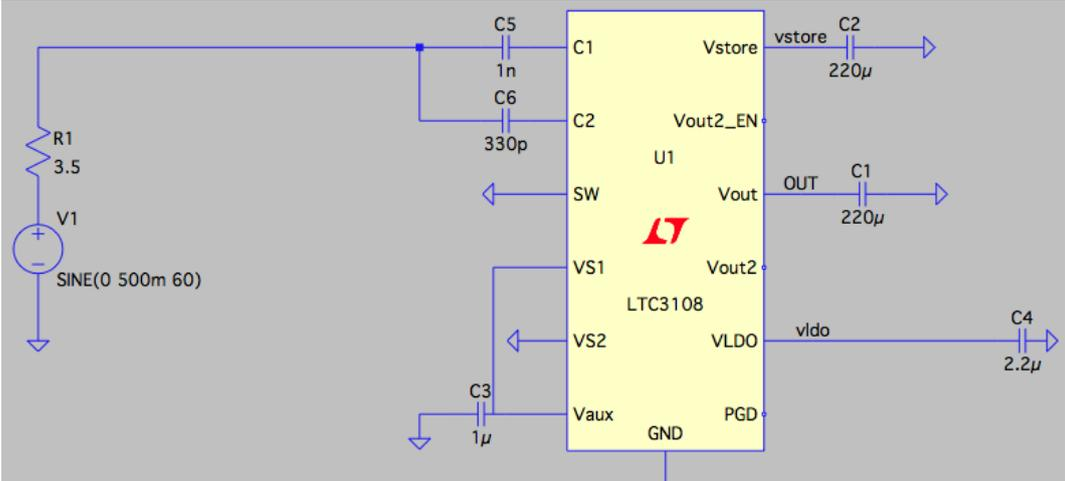
Figure 4.20: Simulation circuit 2
