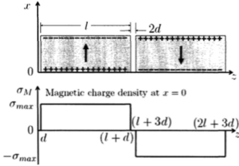
Figure A.4: Schematic of the magnet placement and the resulting charge density on the  $z$ -axis.
