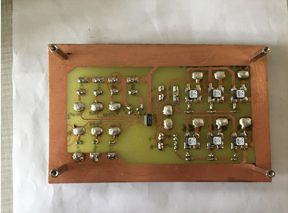
Figure 5.26: Welded Bottom Board for LTC3109
