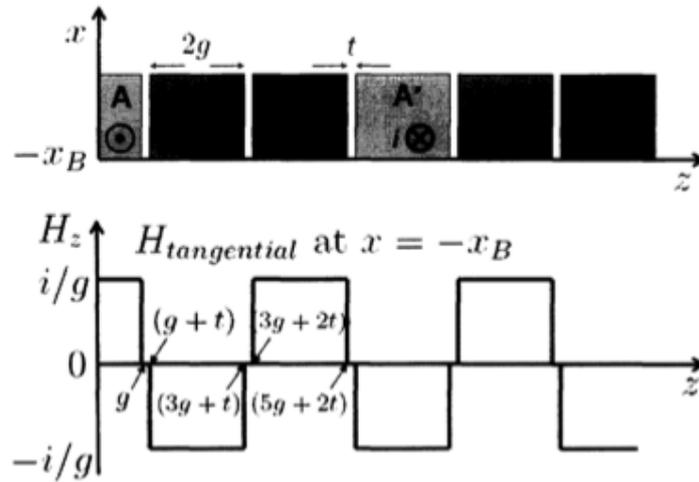
Figure A.5: Schematic of the coil placement and the tangential magnetic field at  $-x_B$  resulting from current  $i$  flowing through all three phases of coils.
