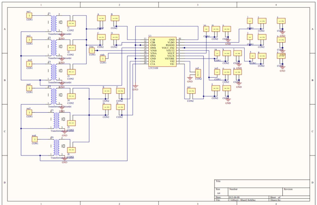
Figure 4.28: Scheme of LTC3109 circuit
