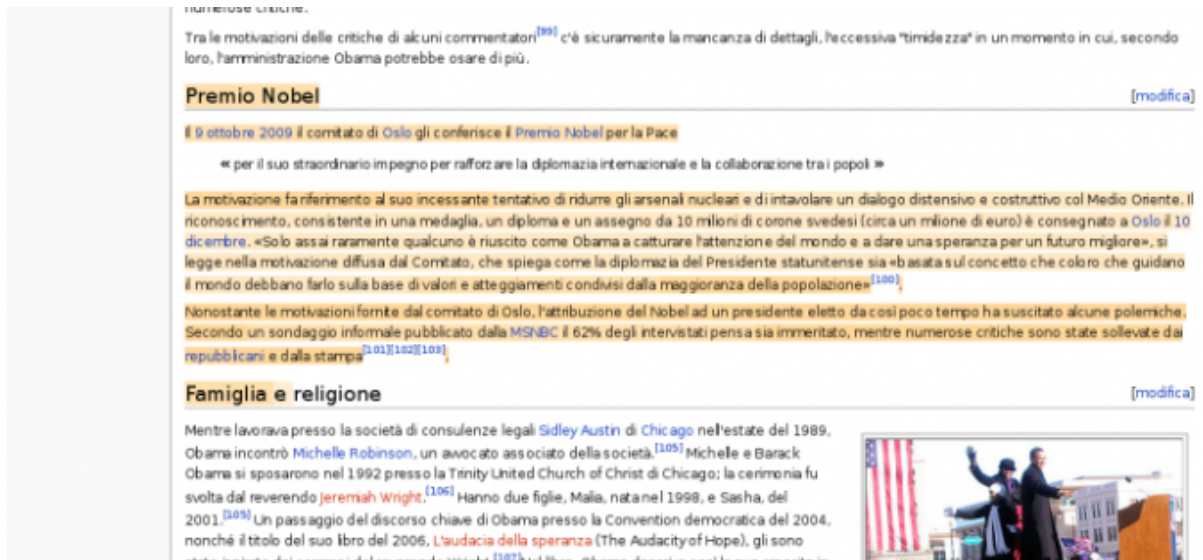
Figure 3.6: Snapshot of the WikiTrust Firefox add-on in action, colouring Wikipedia content according to the reputation metrics computed by the tool.
