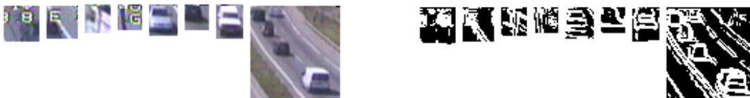
Figura4. Extracted ROIs and Sobel Edge Detector on ROIs
